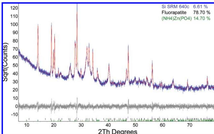
**Figure 2.** XRD/Rietveld analysis of the 50ZnAp sample. Experimental and calculated patterns are shown in blue and red colors, respectively. The Rwp for the fit is 9.1%.
