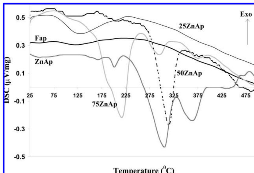
Figure 9. DSC profiles of Zn-containing fluorapatite samples.
