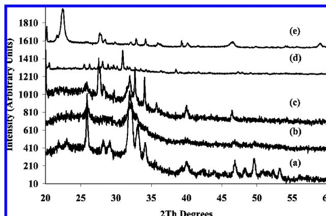
**Figure 1.** XRD patterns of the as-synthesized samples: (a) Fap; (b) 25ZnAp; (c) 50ZnAp; (d) 75ZnAp; (e) ZnAp.**Table 2.** Chemical Phases Identified in the As-Synthesized Samples from Their XRD Patterns
