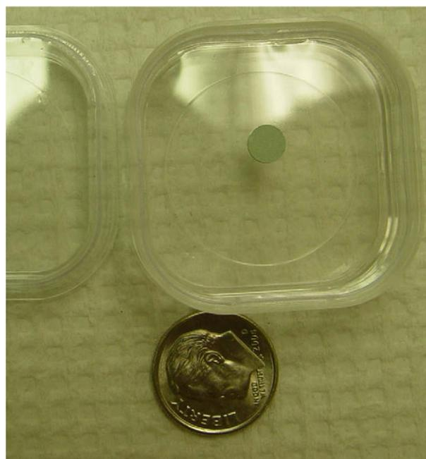
Fig. 1. Picture of sintered plutonium containing zirconia–magnesia inert matrix fuel ( $\text{Zr}_{0.76}\text{Mg}_{0.10}\text{Pu}_{0.078}\text{Er}_{0.062}\text{O}_{1.9}$ ).
